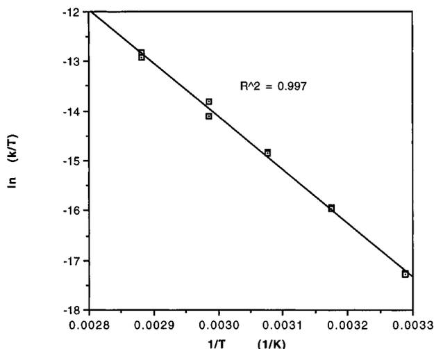
**Figure 3.** Plot of  $\ln(k/T)$  vs  $1/T$  for the formation of  $[\text{N}_3\text{N}]\text{Ta}(\text{C}_6\text{H}_4)$  (**9**) from  $[\text{N}_3\text{N}]\text{Ta}(\text{Me})\text{Ph}$  (**10**) (ten runs; see Experimental Section for a list of individual values).
